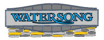
Construction: CNC'd PVC upper structure placed over existing concrete base with stone fascia below. Letters are 2-pc painted PVC. Note: Color rendering shown is a coarse approximation.
